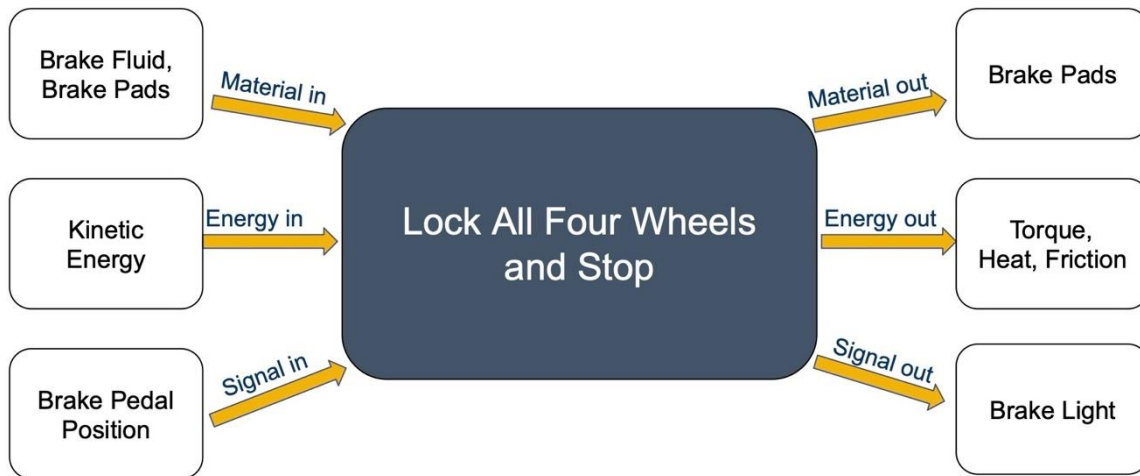
Figure 17: Black Box Model of Brake System
